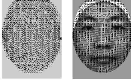
Fig. 2. An example showing pixel-to-vertex map (PVM). AP and IP are expressed as dark and bright pixel in an elliptical mask, respectively.
